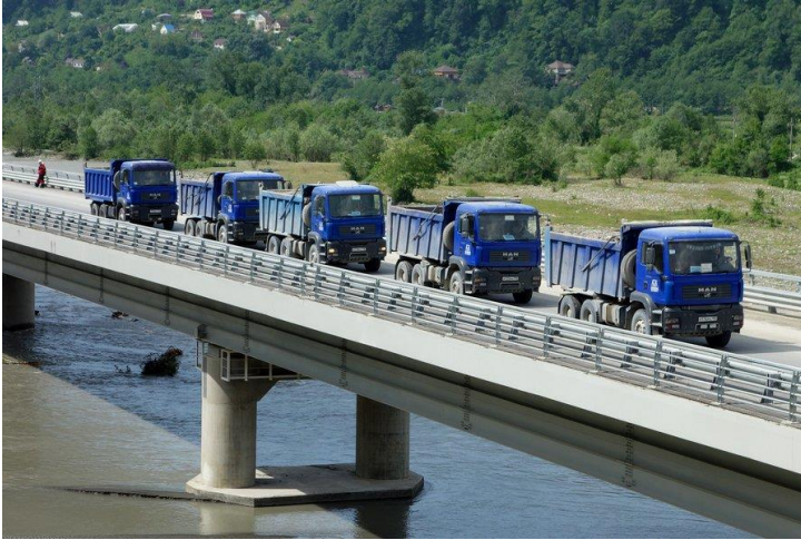
Illustration 3.2. Bridge testing with auto train
