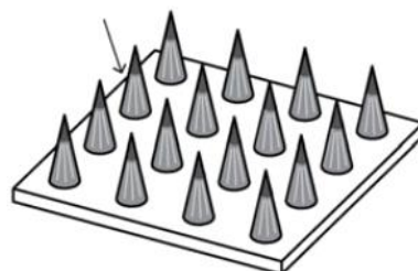
Figure 3 – Heterogeneous wettable cone surfaces
