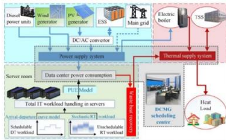
Figure 7 – Microgrid structure diagram of data center
