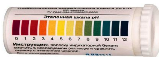
Figure 1.1 – External view of the container with universal indicator paper for determining the pH of the test separating coatings
