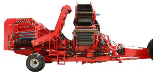
Figure 2 – Hongzhu 4U-90LH potato combine harvester
