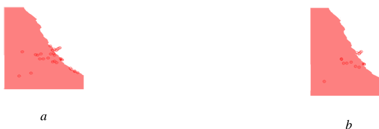
Fig. 1. Before Speckle filter 33 ship target detected with reference to 18 targets (a) and after Speckle filter 15 ship target detected with reference to 18 targets (b)
