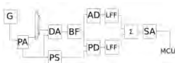
Figure 2 – Block diagram of the device for early anthracosis diagnosis
