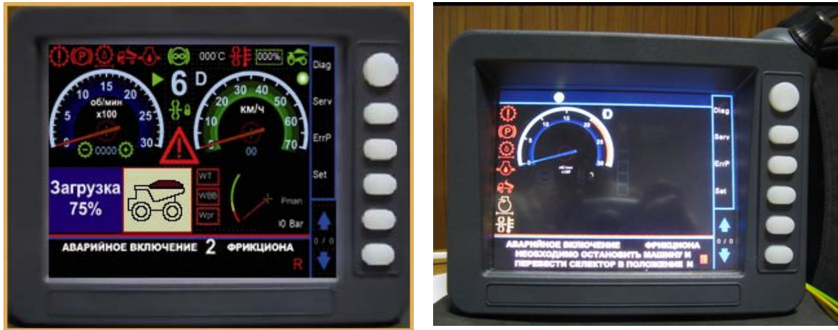
Figure 1: A display MSC HMT company Rexroth Bosch Group: a – general type; b – indication on display one of cut HMT
