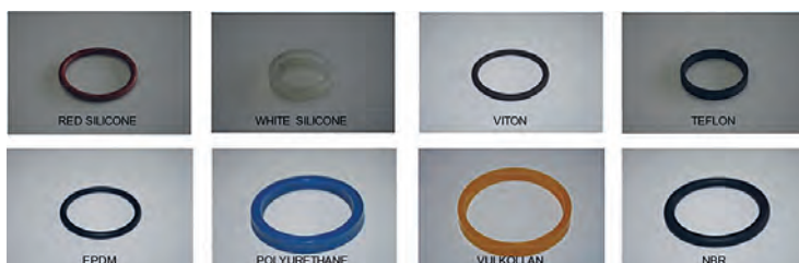
Figure 3. Ecosafe Plus is compatible with elastomers and seals that are generally used in hydraulic systems
