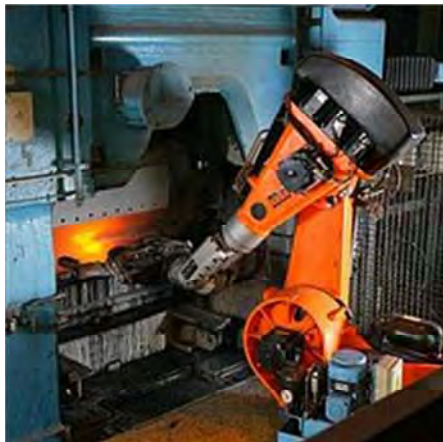
KUKA industrial robot operating in a foundry
