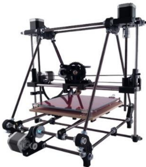
Fig. 1 - Construction of the 3D printer on the basis of Prusa Mendel
