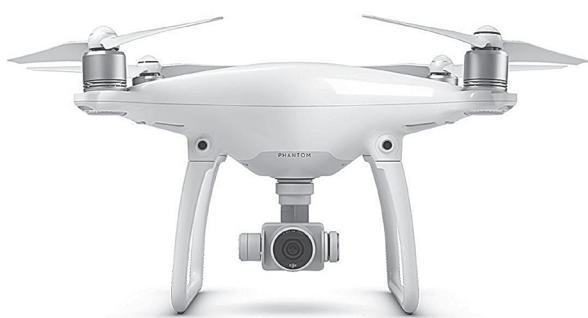
Fig. 4. General View of Phantom-4 Pro Vision Quad-copter as shown in Fig. 4. Its range extender increases Wi-Fi distance to 5 km. Due to its reliability, Phantom-4 Vision Quad-copter use anti-vibration camera platform with single axis stabilization. It operates at low-voltage protection with virtual radar aircraft locator on mobile device. The image processing uses HD Video Recording (H.264 and H.265) and save the sequence of image in JPEG and DNG picture formats and video in MP4/MOV (AVC/H.264; HEVC/H.265) formats. The specifications of Phantom-4 Vision Quad-copter are shown in the Table.
