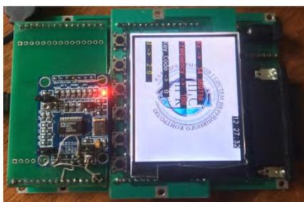
Fig. 1. Model of the developed control system
