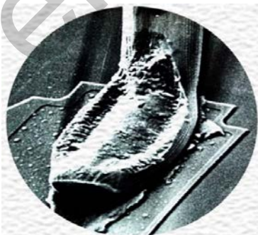
Figure 1 – Typical exterior view of the ultrasonic microbonded wire connection
