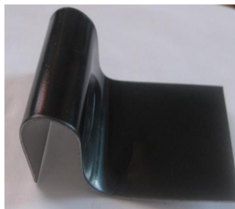
Figure 2. Image of the aluminium plates with decorative films base silica dioxide
