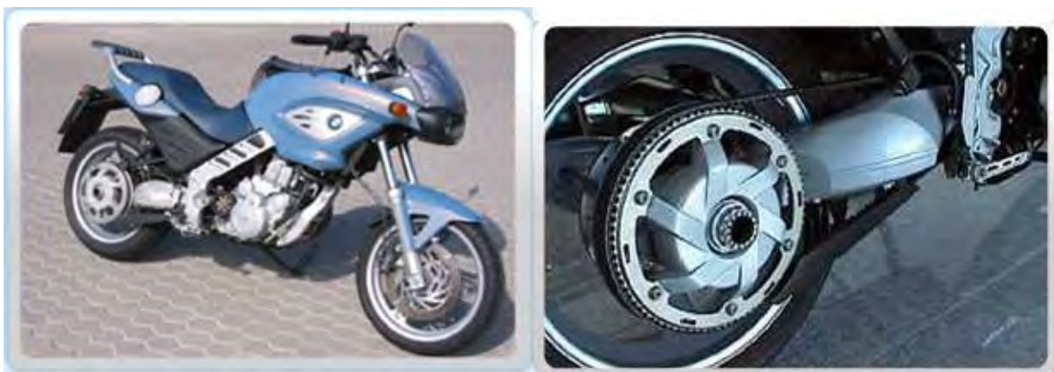
Fig. 1.12. Motorcycle BMW F650 CS with a toothed-belt drive, power of the drive 50 h.p.
