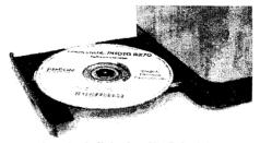
In one type of *optical disk*, the CD-ROM (compact disc read-only memory), digital data is stored as a pattern of tiny pits on a compact disc by the heat of a high-power laser beam or by a stamping machine. Once the information is stored, it can be read but cannot be rewritten. For
