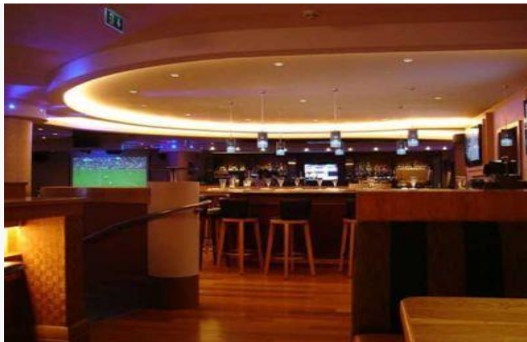
Concealed Lighting / Semi-direct lighting technique
