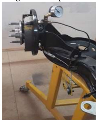
Figure 2 – COBALT car brake system researches stand
