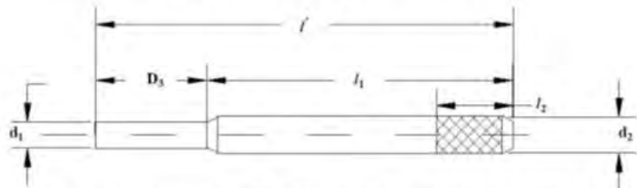
6.2.2.4.a - A typical tommy bar with a holding end.
