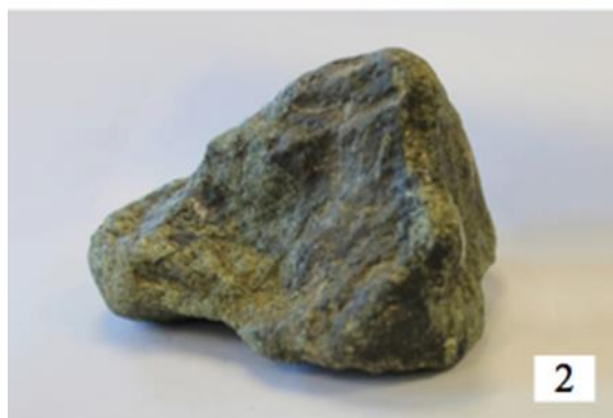
1- pyrite; 2 – chalcopyrite; 3 - halite; 4 – sylvan;
