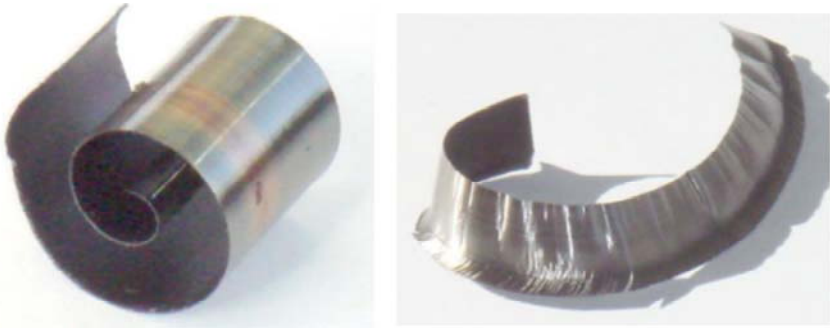
Fig. 9. Shapes of chips obtained in (a) free and (b) non-free cutting
