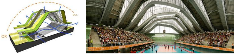
Figure 1.1. Sport center Medellin Columbia – natural ventilation scheme
