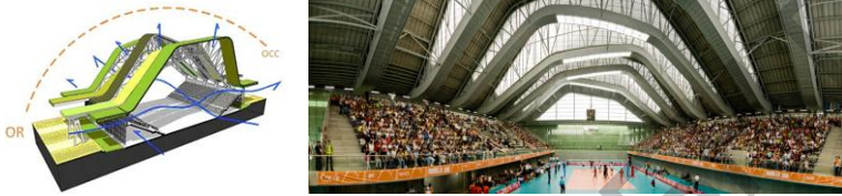
Figure 1.1. Sport center Medellin Columbia – natural ventilation scheme
