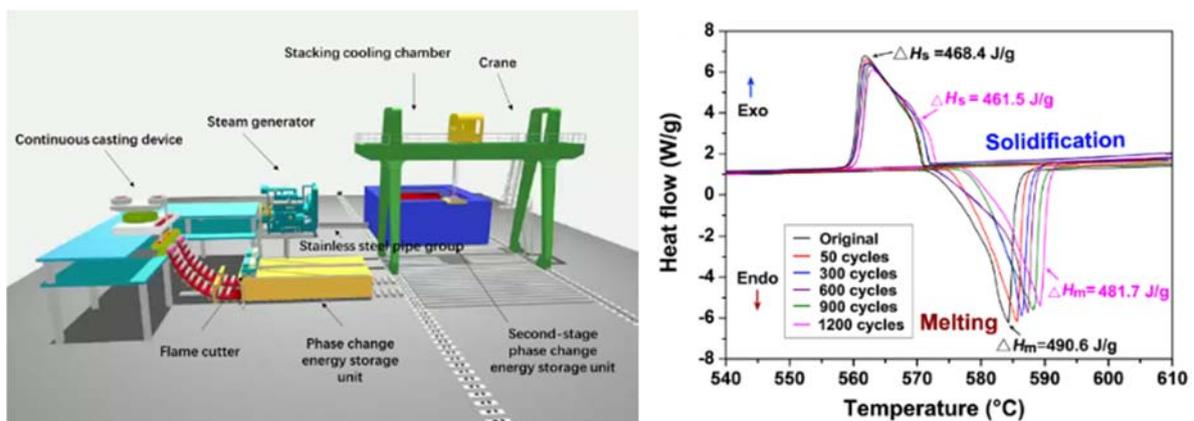
Fig. 2 – Device structure & Thermal cycle simulation results
